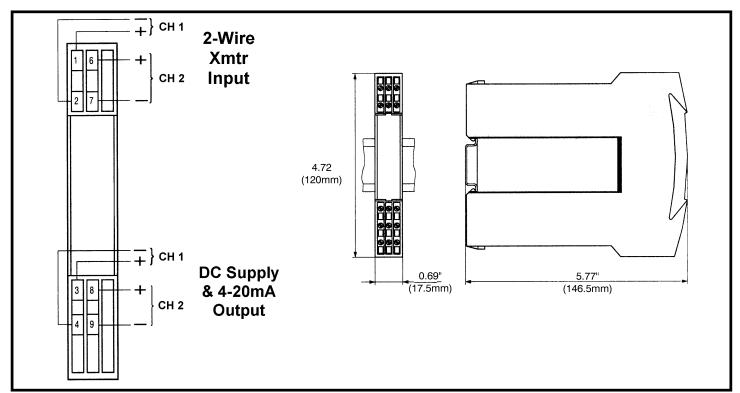
Figure 3: DSCL23-02 Wiring and Dimensions
