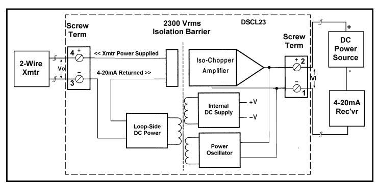
Figure 1: DSCL23-01 Block Diagram, Single Channel Model
