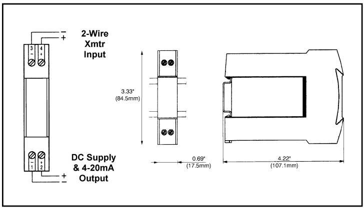
Figure 2: DSCL23-01 Wiring and Dimensions
