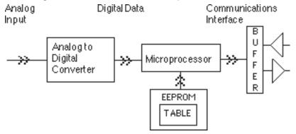
Figure 3. SCM9B-2000 Series Block Diagram
