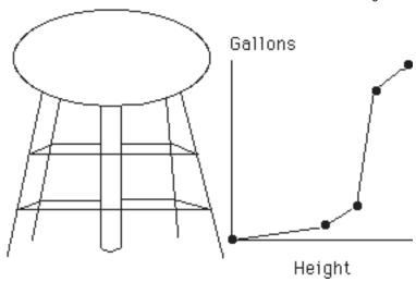
Figure 14. Scaling When Transfer Function is Unknown.
