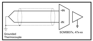
Figure 2: Shield Grounding, Grounded Sensor
