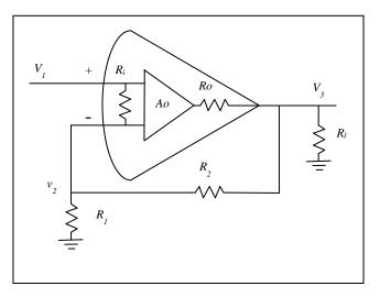
Figure 5 Input and Output Resistance with Load
