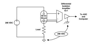
Figure 2 Measurements with High CMV Present
