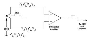
Figure 1 Data Acquisition Differential Operation
