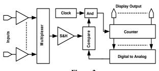
Figure 2 Conceptual ADC System
