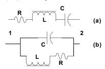
Figure 2 (a) R, L, C in Series (b) R, L in Series, Parallel with C.
