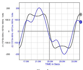
**Figure 2 Fundamental with Third Harmonic Added** Curve 2 170\*Sin(377\*t) +50\*Cos(1131\*t) Curve 1 170\*Sin(377\*t) +50\*Sin(1131\*t)
